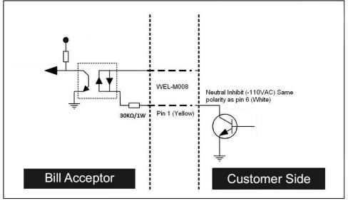
Note: When you use the inhibit line to control the enable/ disable of the BA; the hot enable and neutral enable lines must also be connected or the BA will not enable. The Enable lines can be connected to either 12V DC or 110V AC.
